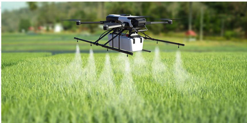
Drone used in Agriculture for spraying pesticides (Credit: Getty Images via Internet)
