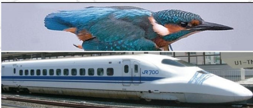
Bullet train design compared to a Kingfisher. Source: Jolie Li, Medium 2021
