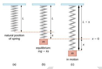
When the particle is displaced from x = 0, the force F tends to draw the particle back towards x = 0. When we pull the spring from x = 0 (say at a displacement x(t) > 0), and releasing, it oscillates up and down. Then according to Newton's second law of motion,
