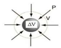
Describes volumetric elasticity or the tendency of an object to deform in all directions when uniformly loaded in all directions. It is defined as volumetric stress over volumetric strain, and is the inverse of compressibility.
