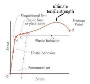
The stress strain graph for a material is as shown in the fig.
