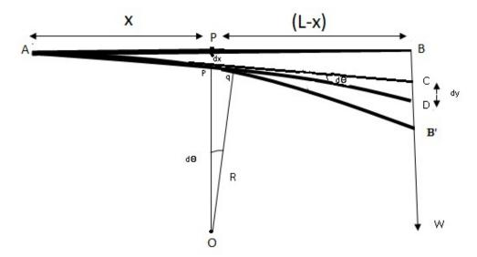
Consider a cantilever of length 'L' fixed at one end and loaded at the other end with a load 'W'. Let AB be the neutral axis of the cantilever. Consider a section P of the beam at a distance 'x' from A as shown in the figure.
