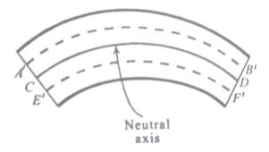
**Neutral surface**: is that layer of a uniform beam which does not undergo any change in its dimension when the beam is subjected to bending within the elastic limit.
