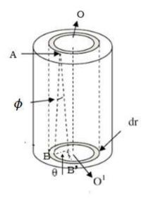
Consider a long cylindrical rod of length 'L' and radius 'R' rigidly fixed at its upper end.
