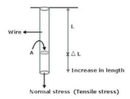
If a bar is subjected to a direct load and hence a stress, the bar will change in length. If the bar has an original length L and changes by an amount  $\Delta L$ , the strain produce is defined as follows:
