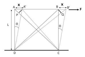
Consider a cube of side 'L', whose lower surface CD is fixed to a rigid support. Let a tangential force 'F' is applied at the upper surface along AB of the cube in a direction as shown
