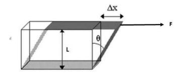
When a body is acted upon by an external force tangential to a surface of the body, the opposite surfaces being kept fixed, it suffers a change in shape of the body, and its volume remains unchanged. Then the body is said to be sheared. The tangential force acting per unit area of the surface is called the 'shearing stress' (F/A).
