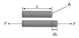
For small change in the length of the wire, the ratio of the longitudinal stress to the corresponding strain is called the **Young's modulus of elasticity (Y)** of the wire.
