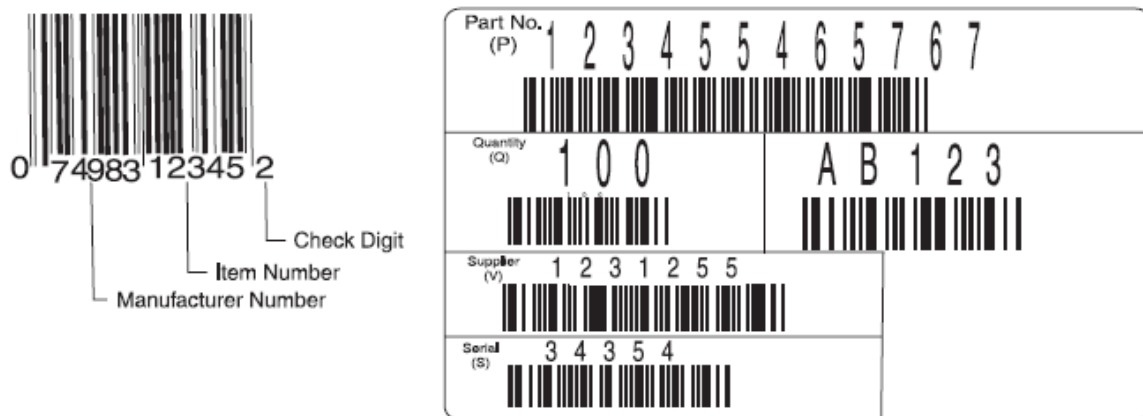
Fig 5.7 (a) Example of universal product code (UPC) format (b) Automotive Industry Action Group (AIAG) format for bar codes
