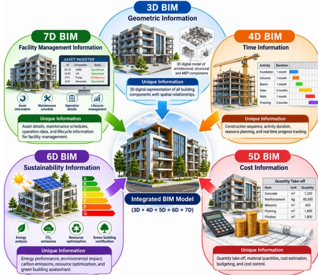
Figure 6: Role of BIM Dimensions (3D–7D) in Developing an Integrated BIM Model Throughout the Project Life Cycle.
